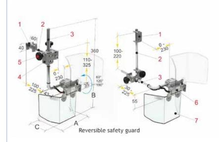
Exclusive item supported by adjustable hexagonal arms. Equipped with a vertically opening shield and with a microswitch integrated in the rotation hinge.
