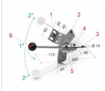
Double-movement universal device, for the insertion of chuck rotation. Provided in a single piece, to be installed as a replacement for one of the two original levers. It allows the activation of chuck rotation, performing a forced "double movement" manoeuvre.
