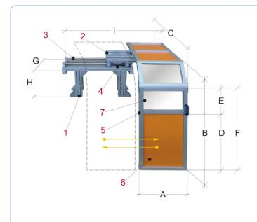
Sliding shield for big sized lathes, designed to be fixed on the machine head, making the whole structure of the guard stable.
