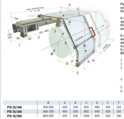
Particularly solid and functional item, designed for the secure protection of the operator against moving parts of the lathe
