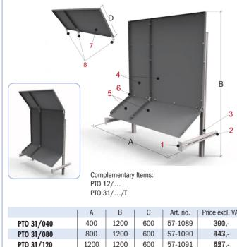
Modular system for rear protection and for shavings containment. Protecting the operator against direct contact with rotating parts accessible from the rear side of the machine and against splashes of lubricants and coolants, as well as against shaving.
