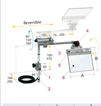
Safety guard with single right-left reversible shield, supported by multi-adjustable hexagonal arms. Equipped with a microswitch integrated in the support hinge.
