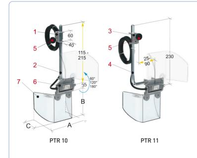
New item proposed with double fixing system, supported by adjustable hexagonal arms. Equipped with microswitch integrated in the rotation hinge.
